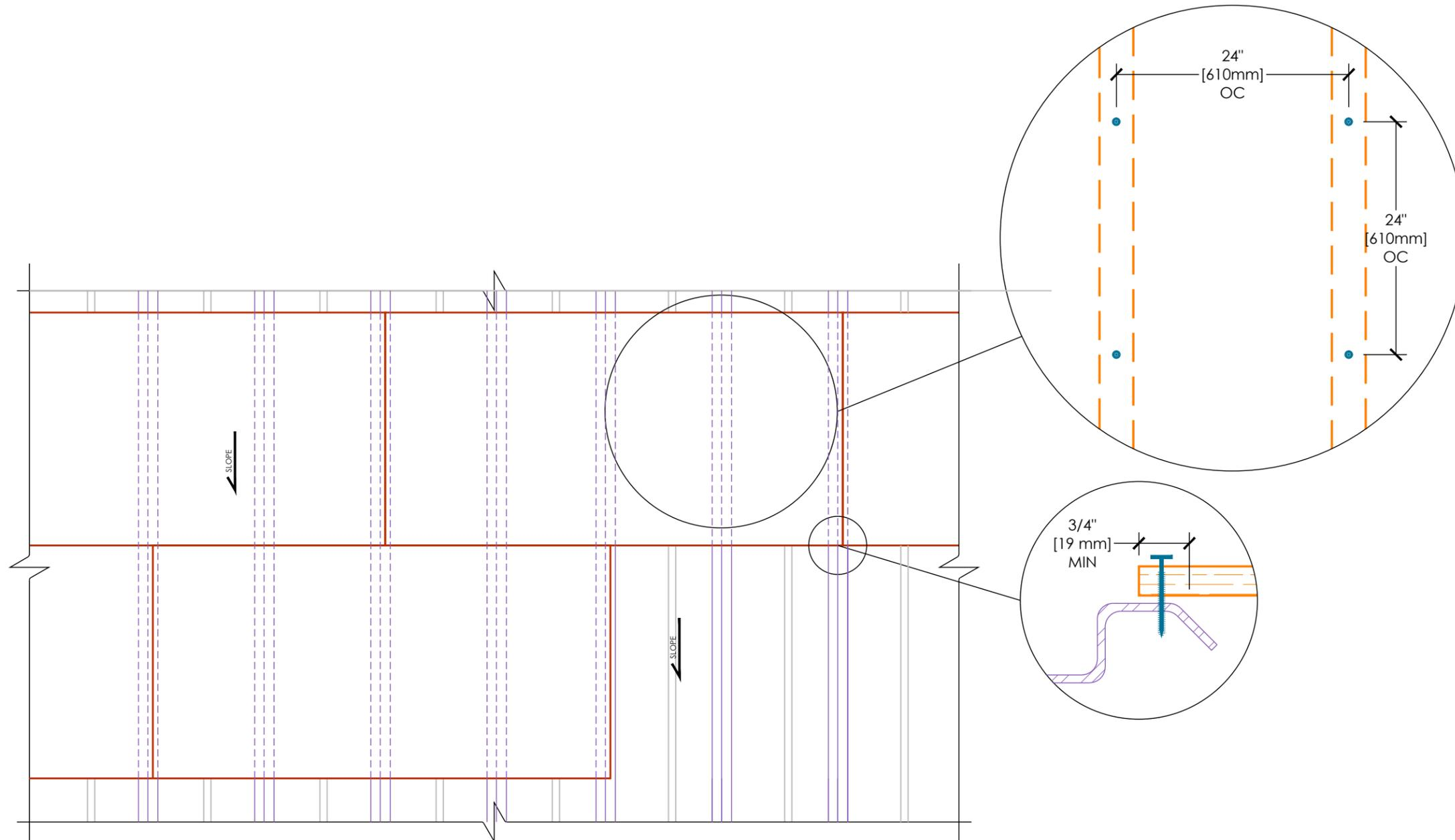
NOTE: MAX BOARD SIZE IS 4' [1219mm] BY 8' [2438mm]. MAX ALLOWABLE GAP BETWEEN BOARDS IS 1/4" [6mm]. STAGGER BOARDS BETWEEN ROWS APPROXIMATELY HALF THE LENGTH OF THE BOARD.
